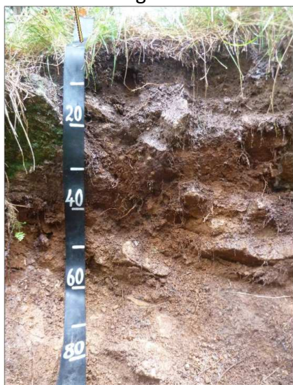
Figure A.6 Trial Hole Depth Readings with Flexible Tape
